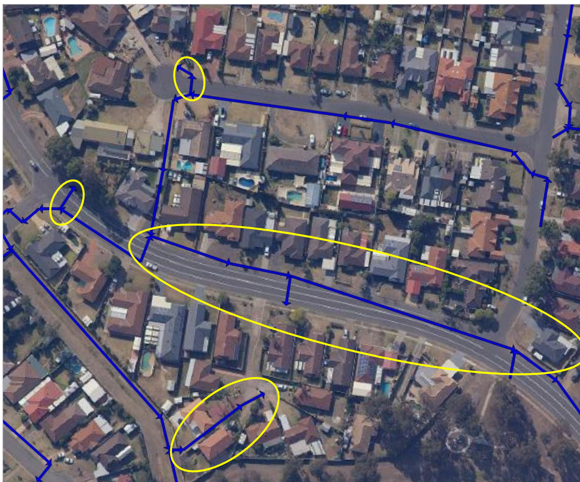
Plate 4 Example of incorrect pipe direction
