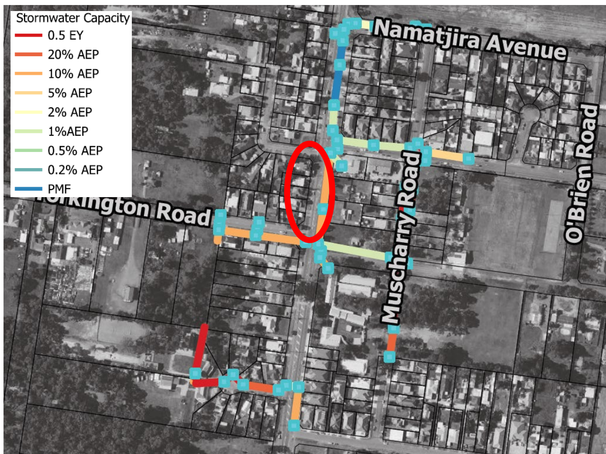
Plate 21 Stormwater capacity in the vicinity of the Carrington Road to Torkington Road hotspot.
